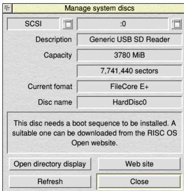
**Figure 5 - Completed operation, awaiting !Boot application**
